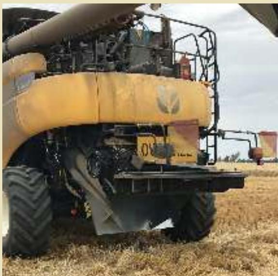
**Figure 4.** Narrow windrow chute fitted to harvester, Wolseley 2017
