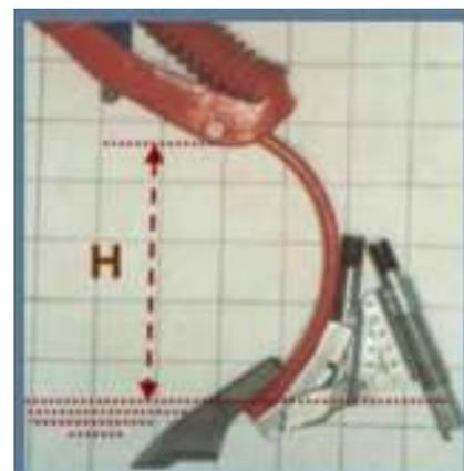
**Figure 3.** Vertical Tyne Clearance. (Courtesy of J.Desboilles, University of SA)
