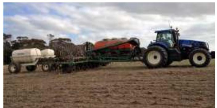
Figure 1. DBS Seeder Sowing into Stubble
