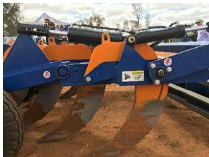
Figure 9b. Grizzly Deep Digger with parabolic tines.
