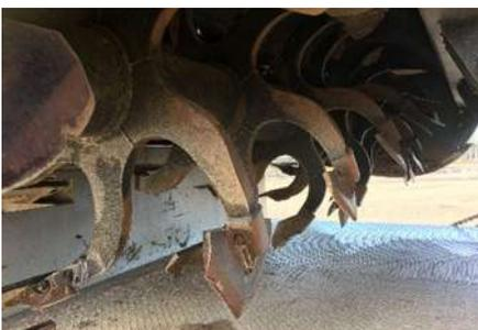
Figure 10a. Triangular shaped spades on curved tines are fixed to a central shaft that rotates at ~90 revs/min<sup>10</sup>.
